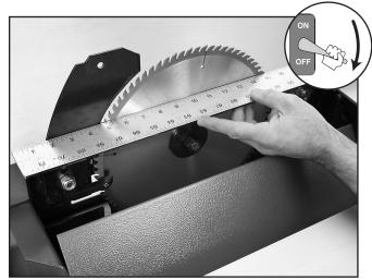
Figure 37. Checking riving knife alignment.
